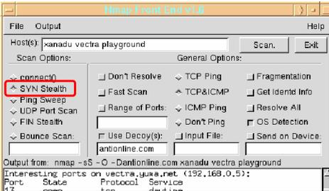
The screenshot shows the Nmap Front End v1.8 interface. The 'SYN Stealth' option is checked and highlighted with a red box. The output window shows the results of the scan on 192.168.0.5.
