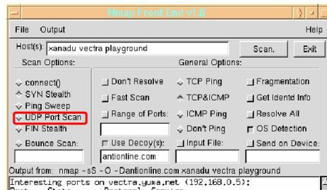
The screenshot shows the Nmap Front End v1.8 interface. The 'UDP Port Scan' option is checked and highlighted with a red box. The output window shows the results of the scan on 192.168.0.5.
