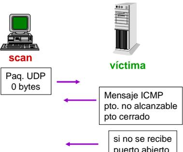
The diagram shows a 'scan' host sending a UDP packet (0 bytes) to a 'víctima' (victim) host. If the victim responds with an ICMP message indicating the port is unreachable, it is labeled 'Mensaje ICMP pto. no alcanzable pto cerrado'. If no response is received, it is labeled 'si no se recibe puerto abierto'.
