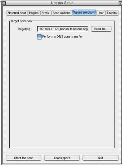
The screenshot shows the 'Target selection' tab in the Nessus Setup window. The 'Target(s):' field contains '192.168.1.1/29,bonsai.fr,nessus.org'. There is a 'Read file...' button to the right. Below the field, there is a checkbox labeled 'Perform a DNS zone transfer' which is currently unchecked. At the bottom of the window, there are three buttons: 'Start the scan', 'Load report', and 'Quit'.
