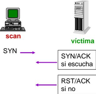
The diagram shows a 'scan' host sending a SYN packet to a 'víctima' (victim) host. If the victim responds with SYN/ACK, it is labeled 'si escucha' (it listens). If it responds with RST/ACK, it is labeled 'si no' (if not).
